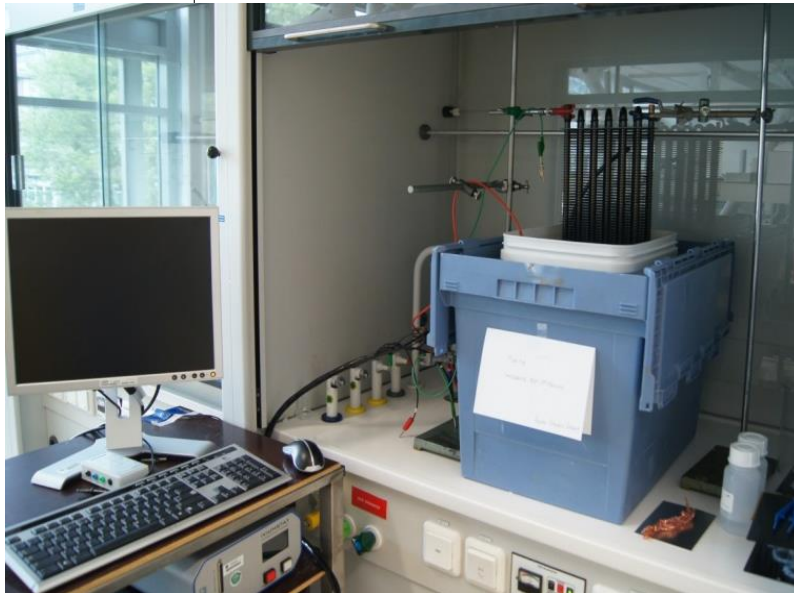
Large set-up for immersion of whole HX = 60 \times 20 \times 5\text{cm}^3 (!)
